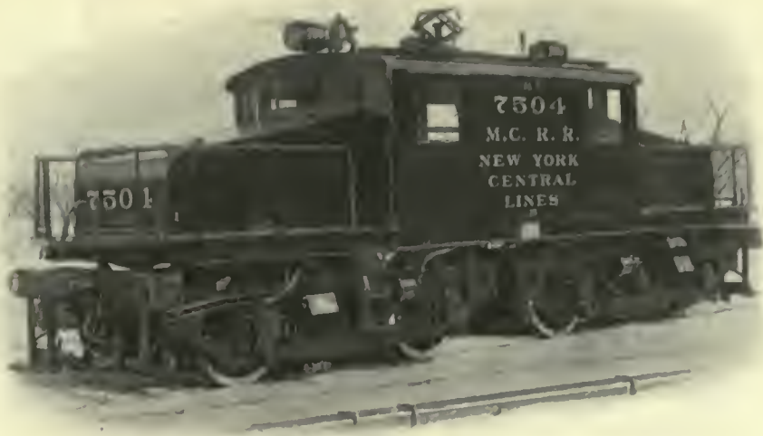
FIG. 532. ELECTRIC LOCOMOTIVES. Electric Locomotive for 600-Volt Direct Current Third Rail Operation, Michigan Central Railroad.
